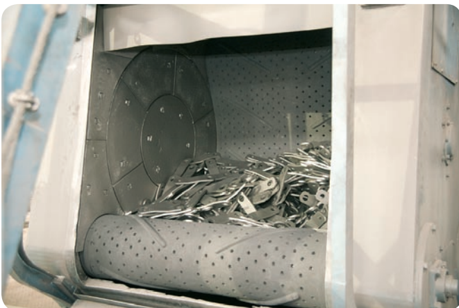
Shot peening improves fatigue strength and crack resistance
